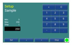
The numeric input consists of the buttons **Set** / < / > / **Exit**, a numeric keypad and the parameter display. The meaning of the buttons:
