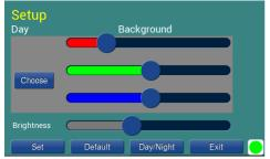
The configuration allows to define two colour styles. The settings are called "Day colours" and "Night colours" in the set-up. The settings take effect immediately. Background and button colours can be changed. The brightness can be adjusted, but is the same for both.
