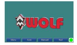
As long as no measurement data is available, the logo is displayed in the background. If measurement data is available, the last measurement value and the statistical values of the last measurement series are displayed. Operation display (bottom-right) shows the current status of the measuring device. (Green -> ready for a measuring task / Red -> measuring device is in an active measurement)
