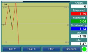
This is the access point for manual measurement. The individual measurement is triggered with Start (or by pressing the foot-operated switch). The display is graphical and numerical. The scaling works as described for the automatic measurement. To return to the main menu, press "Exit".
