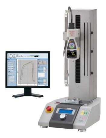
The FSA series is a unit for forcedisplacement measurement including force gauge, test stand, cable and software.
