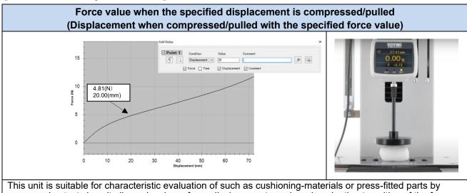
This unit is suitable for characteristic evaluation of such as cushioning-materials or press-fitted parts by compression test since it allows drawing a force-displacement graph and evaluating transition of the force value to the compressed displacement. Also, as you see in the picture above, it enables you to easily search for the force value at a specific displacement value on the graph and leave a comment.
