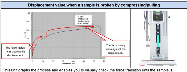
broken. Also, it helps you to easily find the force/displacement value and peak value when the sample is broken, and leave a comment.
