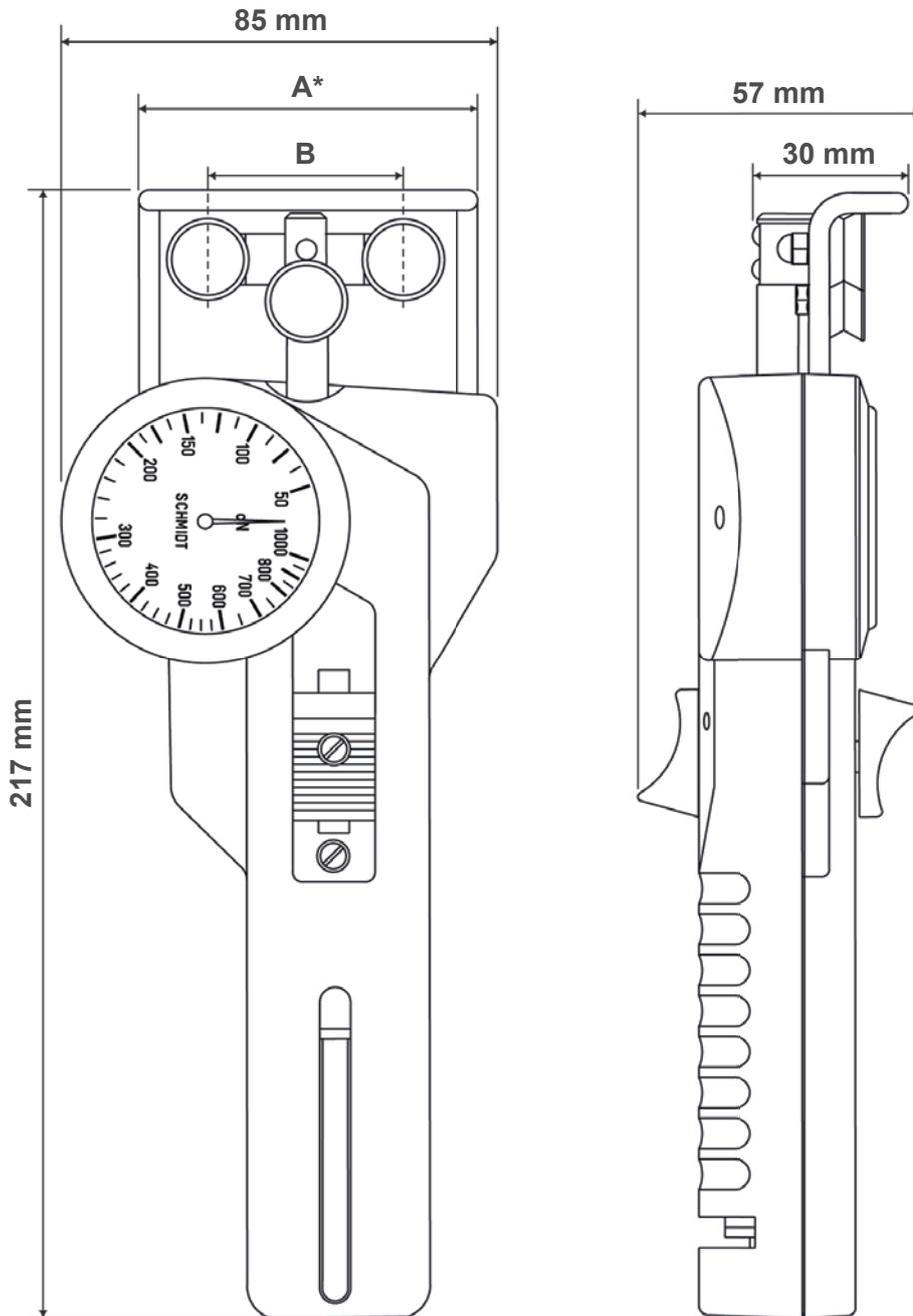
\*The measuring head width is depending on the width of filament guide or outer distance between outside guide rollers respectively.
