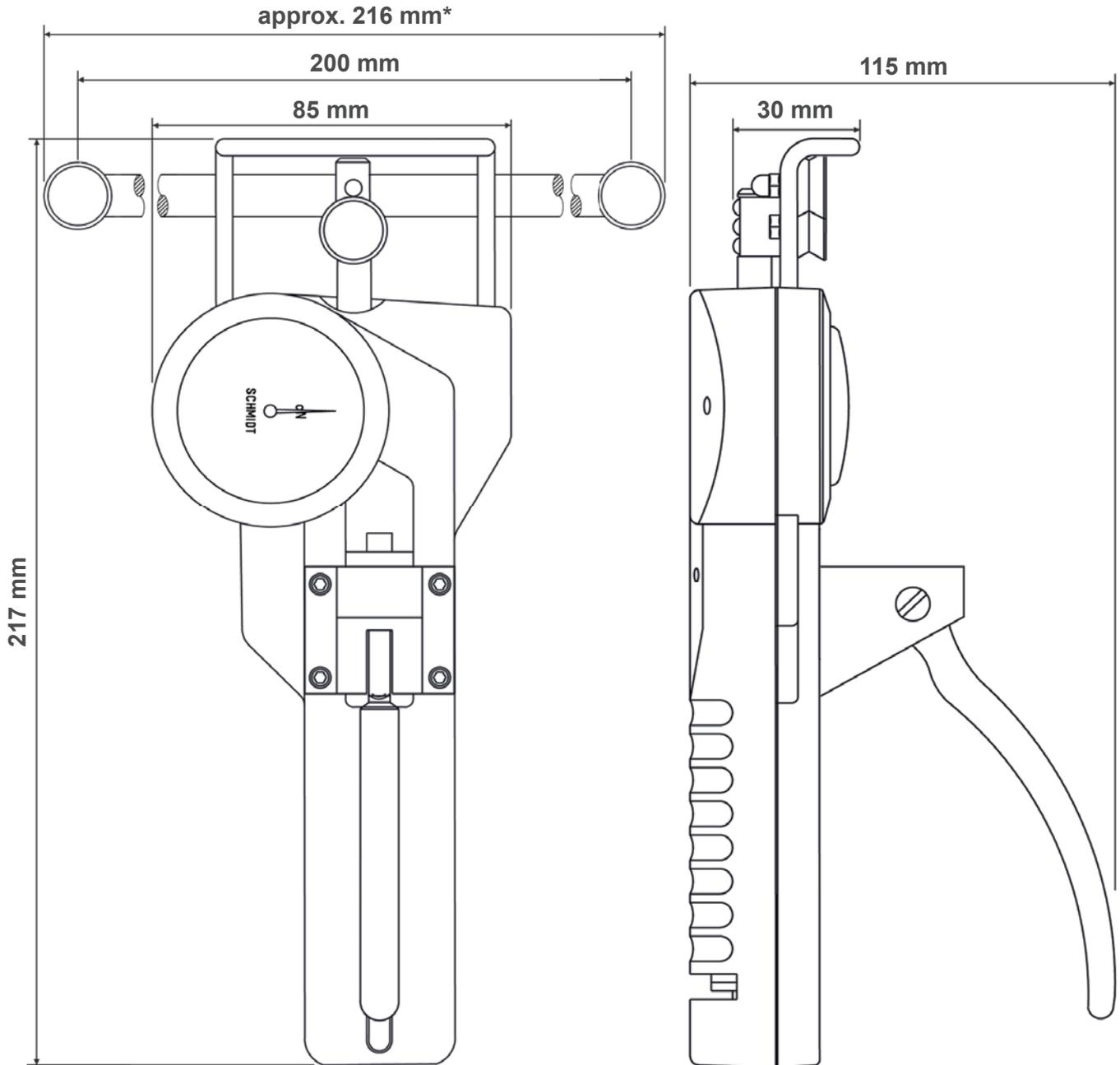
\*The measuring head width is depending on the outer distance between outside guide rollers.
