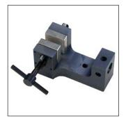
Vice grip for clamping paper, foil, fabric etc. **max. load 1 kN**, clamping size 30 x 30 mm delivery includes 1 pair (2 pieces) without jaws *Order number: TH56k*
